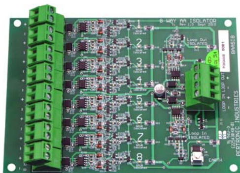
Analogue Addressable Isolator Board – 8 Spur (8SAAIB)
