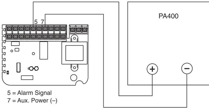
**Figure 12. Insulator Card for DH200RPL Duct Smoke Detector**
