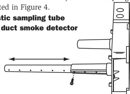
**[4.1] Installation For Ducts Greater Than 1½ Feet (0.46m) But Less Than 8 Feet (2.4m) Wide**
