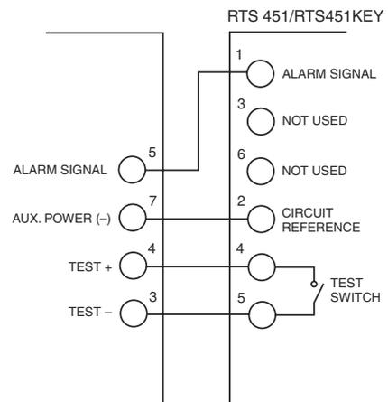
FOR RTS451, TERMINAL 1 IS NOT USED. (RTS451 DOES NOT HAVE A TERMINAL 6.) FOR RTS451KEY, TERMINALS 3 AND 6 ARE NOT USED.
