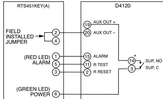
\* Sup. contacts cannot be used if they are wired to control panel.
