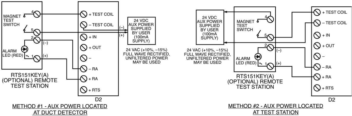
**NOTE: THE USE OF THE RTS151KEY(A) REQUIRES THE INSTALLATION OF AN ACCESSORY COIL, DCOIL, SOLD SEPARATELY.**
