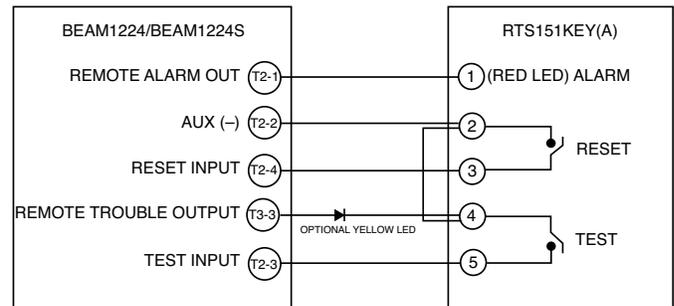
NOTE: RTS151KEY(A) CAN BE USED WITH INTELLIGENT BEAM DETECTOR PRODUCTS. CONSULT INTELLIGENT BEAM DETECTOR MANUAL FOR ADDITIONAL INSTRUCTIONS
