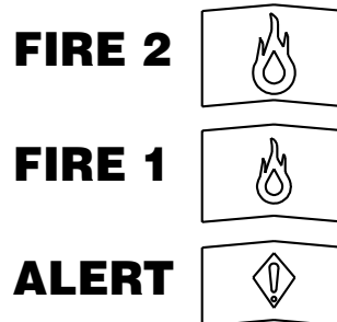
FIGURE 7. ALARM LEVEL DISPLAY
