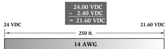
The voltage at the last device will be 21.6 VDC which is within the operating range of the devices used and satisfies the minus 10% rule mentioned above. Remember, it is still necessary to ensure the power supply is capable of supplying the necessary electrical current for the notification appliances.
