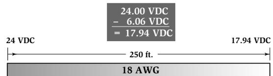
The voltage at the last device would be 17.94. Obviously, this is not within the range for the notification appliance to function properly. If 14 AWG solid copper wire is used instead of 18 AWG, the voltage drop changes to:
