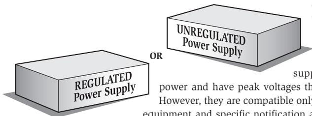
Unregulated power supplies provide DC power and have peak voltages that may be very high. However, they are compatible only with specific control equipment and specific notification appliances. It is therefore important to verify with the fire panel manufacturer or
