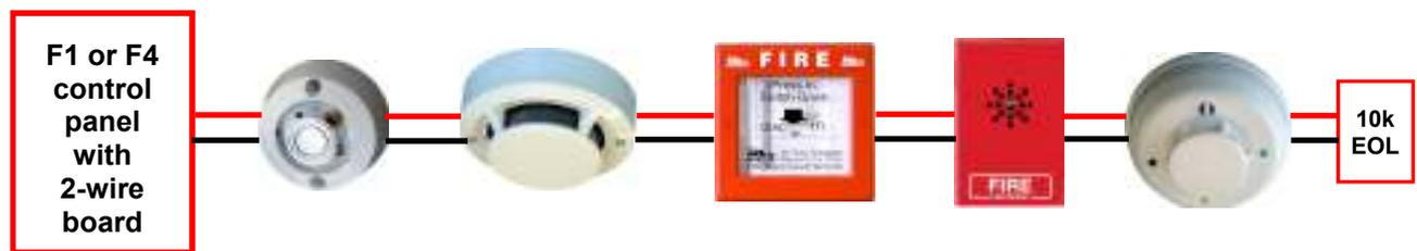
The diagram above shows the range of devices that can share the common detector/sounder circuit - from the control panel end; a heat detector, smoke detector, manual call point, PS1 sounder, 2WTA-B detector/sounder. The 2WTA-B is a photoelectric smoke & thermal detector with an inbuilt sounder that further simplifies installation by removing the need for separate sounders.
