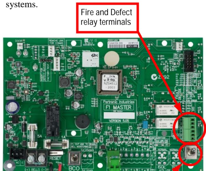
The new F1 fire alarm panel master PCB (version 5.x)
