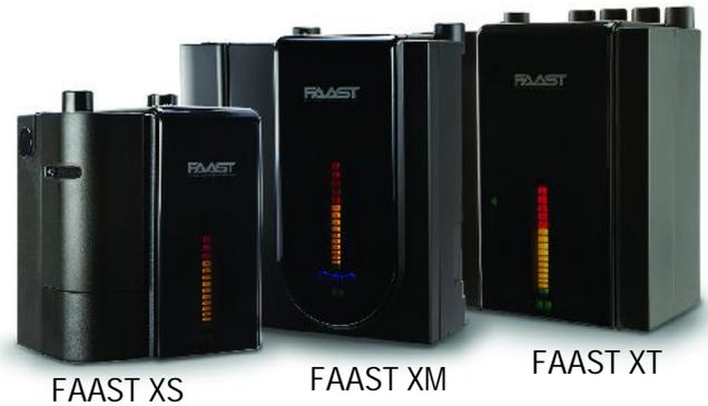
Designed for maximum sensitivity without compromising nuisance alarm immunity, the dual-vision aspirating smoke detectors from System Sensor USA feature a particle separator that removes large, non-fire particles, keeping the internal sensing chamber clean and extending the life of the replaceable filter. The software combines signals from two separate optical sensors (blue LED and infra-red laser) to reliably detect smoke as thin as 0.0015 % obscuration per metre.
