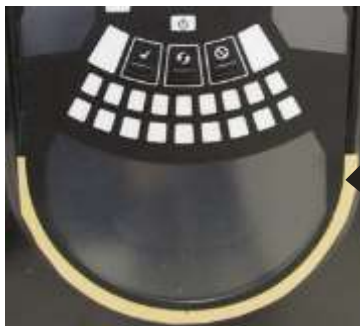
Figure 3: Remove backing tape to stick cover down
