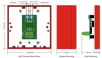
To prevent damage to the PCB, care MUST be taken to ensure cables do NOT come between the PCB and the back of the enclosure.
