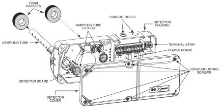
efficient housing design that samples air passing through a duct and allows detection of a developing hazardous condition. When sufficient smoke is sensed, an alarm signal is initiated at the fire control panel monitoring the detector, and appropriate action can be taken to shut off fans, blowers and change over air handling systems, etc. This can prevent the distribution or it can isolate toxic smoke and fire gases throughout the areas served by the duct system.
