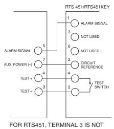
FOR RTS451, TERMINAL 3 IS NOT USED. (RTS451 DOES NOT HAVE A TERMINAL 6.) FOR RTS451KEY, TERMINALS 3 AND 6 ARE NOT USED.
